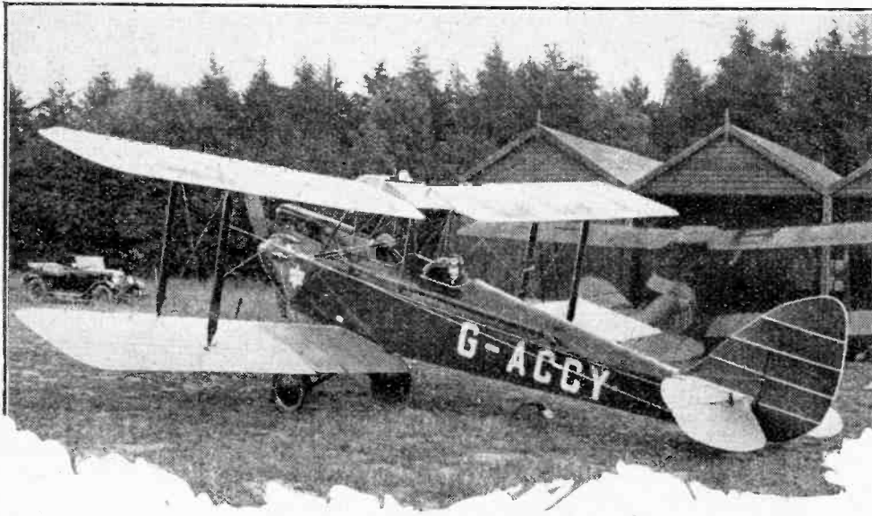
The Gypsy Moth ready for the start. The aerial can be seen slung between the left rear strut and the tail plane.
